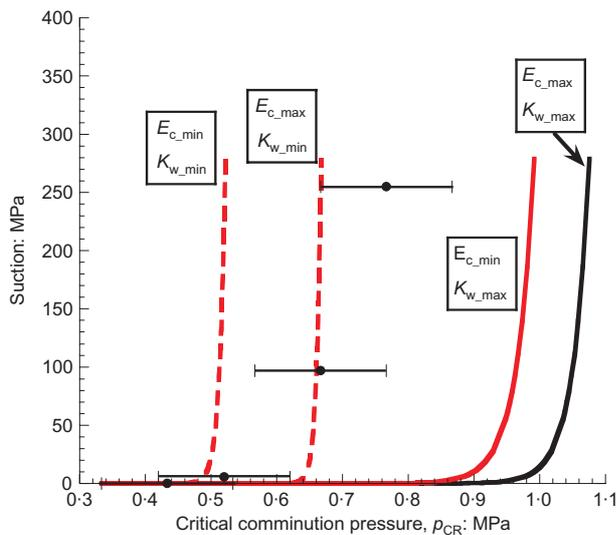
**Fig. 11. Comparison of theoretical critical comminution pressures against experimental data for Pancrudo rockfill (data after Oldecop & Alonso, 2003) (error bars represent experimental data; continuous lines model predictions)**
