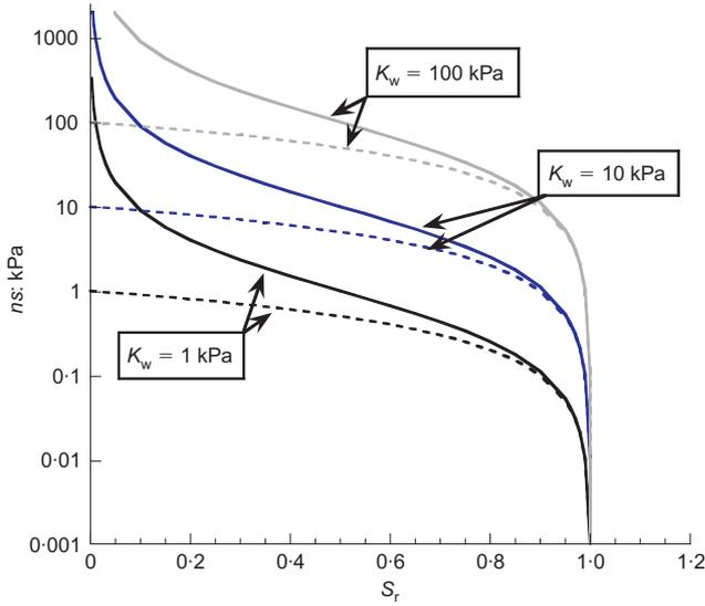
**Fig. 1. Schematic plot of the two alternative water retention curves in the  $ns$ - $S_r$  plane (dotted lines represent linear retention curve; continuous lines represent hyperbolic retention curve)**
