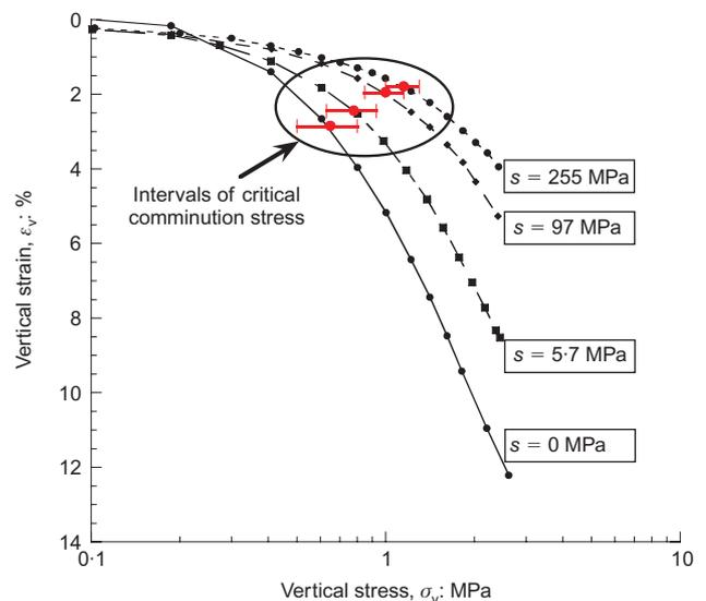
**Fig. 10. Yielding upon oedometric loading: stress–strain curves (redrawn after Oldecop & Alonso, 2003)**
