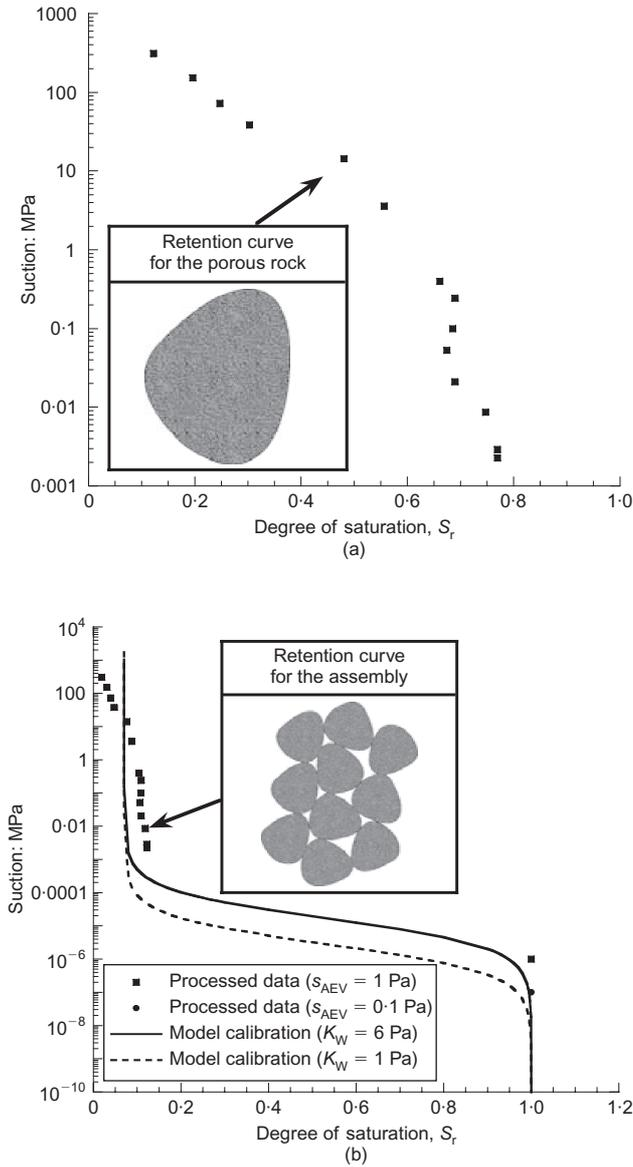
**Fig. 9. (a) Water retention data for Pancrudo slate; (b) processed data and model calibration for granular assembly (residual degree of saturation  $\bar{S}_r = 0.07$ ; total porosity  $n = 35\%$ )**
