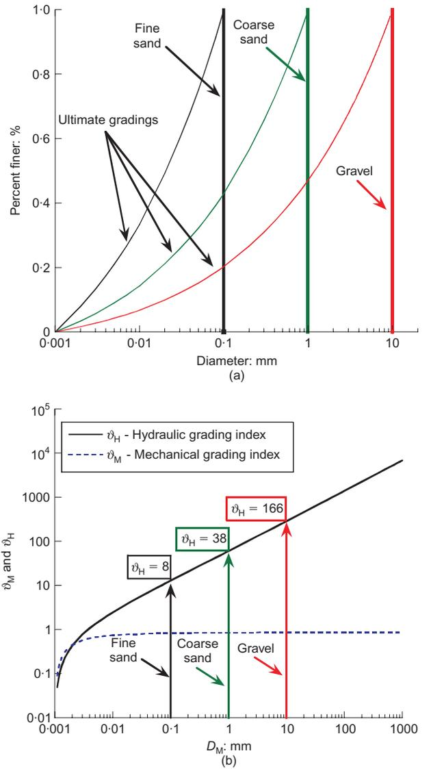
**Fig. 5.** (a) Examples of initial and ultimate grading curves for different granular materials; (b) dependence of  $\vartheta_M$  and  $\vartheta_H$  on maximum grain size for uniform initial GSD
