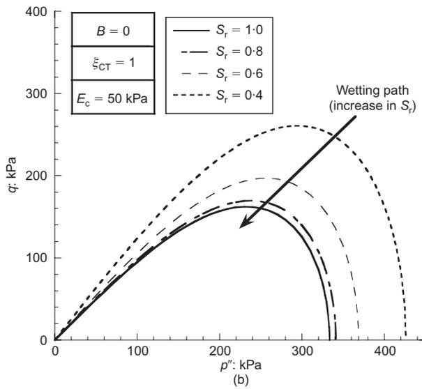
**Fig. 7. Evolution of yield surface with  $S_r$  on the  $p''$ - $q$  plane: (a) linear retention curve ( $\xi_{CT} = 1$ ); (b) hyperbolic retention curve ( $\xi_{CT} = 1$ )**
