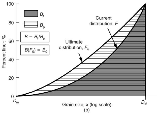
**Fig. 2. Definition of breakage: (a) dependent on initial GSD; (b) universal definition as a function of  $D_M$  (see Einav, 2007a, for further discussion of the applicability of the universal definition)**
