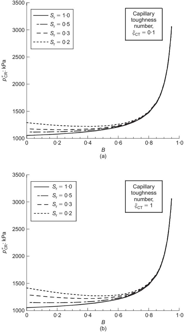
**Fig. 6. Evolution of critical comminution pressure with  $B$  for different values of  $S_r$ : (a) linear retention curve; (b) hyperbolic retention curve. Figure illustrates the possibility for transition from softening to hardening for lower values of  $S_r$ .**
