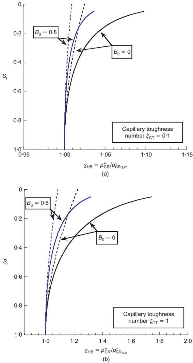
**Fig. 4.** Description of increase in isotropic yield limit with partial saturation: (a)  $\xi_{CT} = 0.1$ ; (b)  $\xi_{CT} = 1$  (dotted lines represent linear retention curve; continuous lines represent hyperbolic retention curve)
