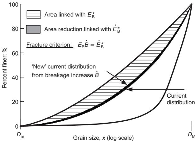
**Fig. 3. Graphical interpretation of energetics of particle breakage: incremental breakage dissipation is equal to incremental change in residual breakage energy (Einav, 2007c). Similar interpretation follows when breakage is defined using the universal GSD (i.e. in alteration according to Fig. 2(b))**
