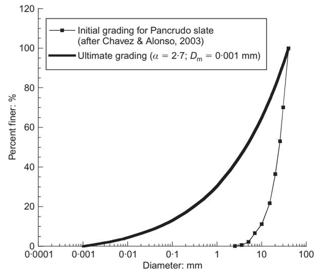
**Fig. 8. Initial and ultimate grading curves for Pancrudo slate**
