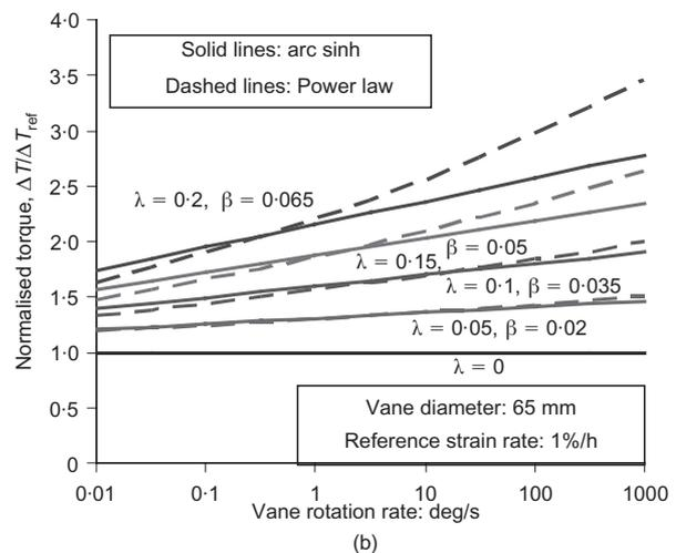
Fig. 4. Effect of vane rotation rate on torque: (a) comparison of arc sinh and simple model; (b) comparison of arc sinh and power law models
