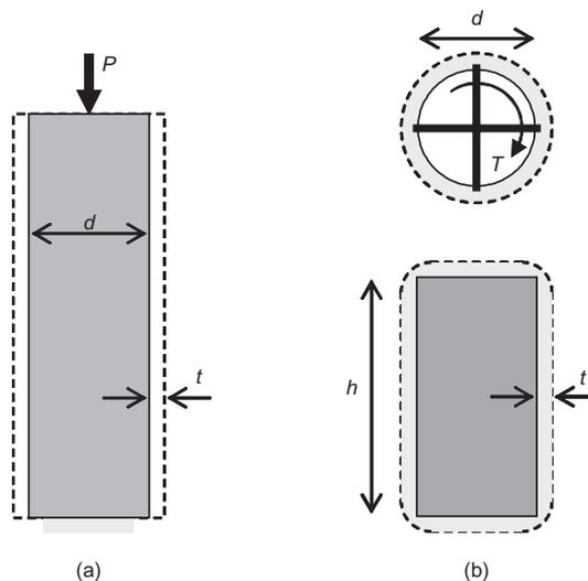
Fig. 1. Schematic of cylindrical shear bands: (a) pile under axial loading; (b) vane undergoing torsion
