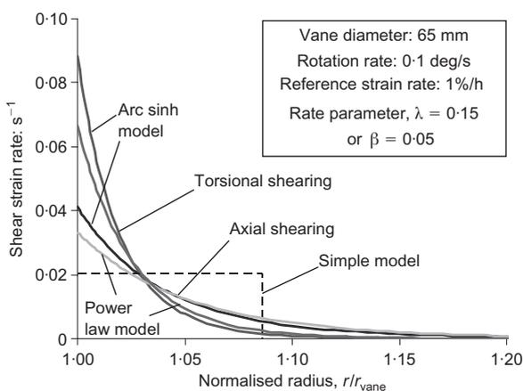
Fig. 3. Profiles of shear strain rate within shear band for all three models
