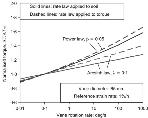
Fig. 5 Comparison of rate laws applied to soil or directly to vane torque
