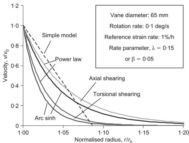
Fig. 2. Velocity profiles within shear band for all three models
