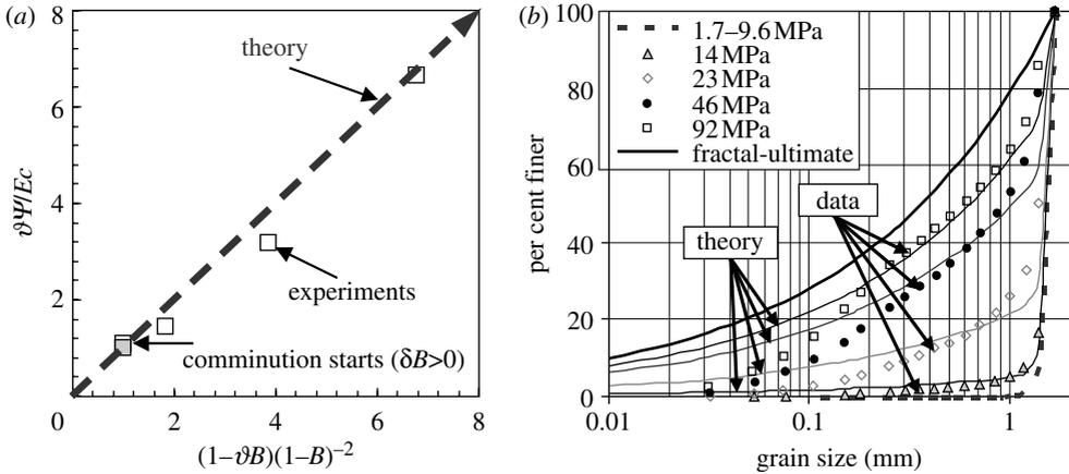
Figure 6. Theoretical (Einaev 2007c) versus experimental (Nakata *et al.* 2001) relation between the vertical stress and breakage in one-dimensional compression of silica sand: (a) breakage hardening (dashed line is the arrow of time) and (b) the corresponding evolving gsd.
