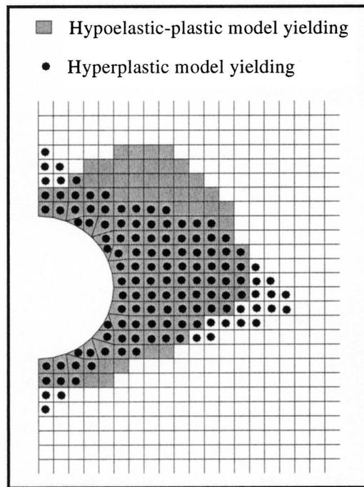
**Fig. 10.** Close-up view on yielding region for  $H/D=3.5$  (for first set of parameters  $\bar{G}=103$  and  $n=1$ )
