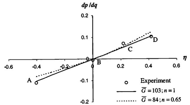
Fig. 4. Variation of  $dp/dq$  with stress ratio  $\eta = q/p$
