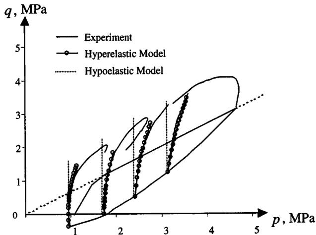
Fig. 5. Model's prediction of undrained triaxial test
