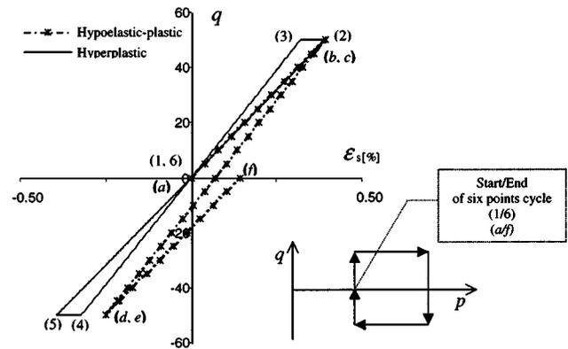
**Fig. 2.** Stress-strain curves for closed-loop stress path [hypoelastic-plastic model numerated by (a,b,...) and hyperplastic model numerated by (1,2,...)]
