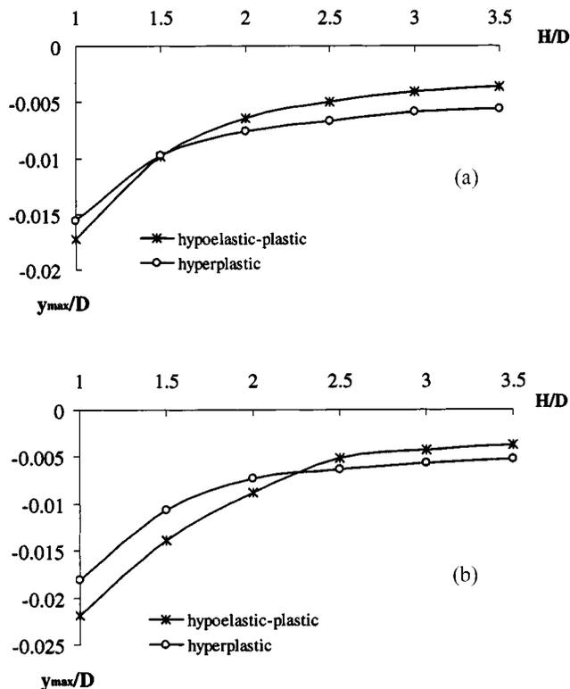
**Fig. 8.** (a) Normalized maximum-settlement of ground surface (for the first set of parameters  $\bar{G}=103$  and  $n=1$ ) and (b) normalized maximum-settlement of ground surface (for the second set of parameters  $\bar{G}=84$  and  $n=0.65$ )
