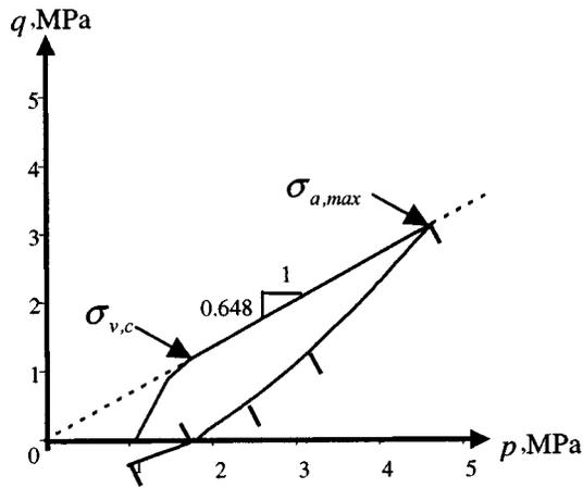
Fig. 3. Stress path prior to undrained shearing (Borja et al. 1997)
