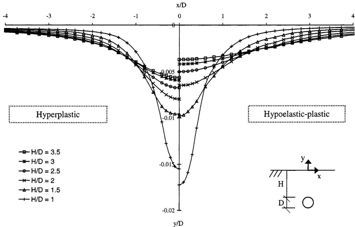
Fig. 7. Normalized settlement troughs at ground surface for different  $H/D$  ratios (for first set of parameters  $\bar{G}=103$  and  $n=1$ )
