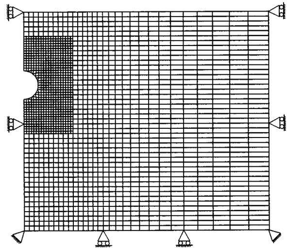
Fig. 6. Typical finite-element mesh
