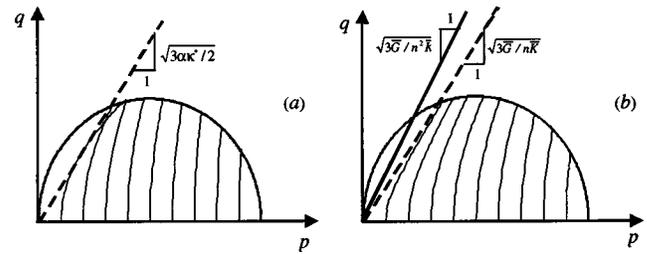
Fig. 1. Undrained stress paths for elastic behavior inside yield locus: (a) Houlsby (1985) and (b) new function (for  $n = m = 0.65$ )
