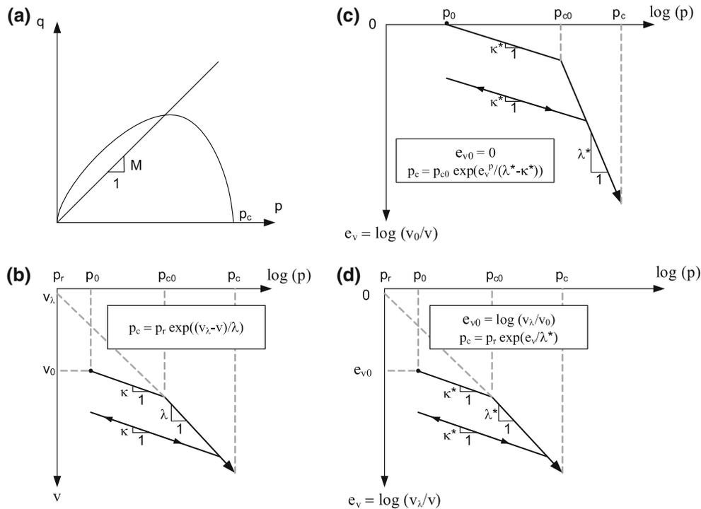
**Fig. 4** a Typical yield surface projection in stress-space, **b–d** three alternative definitions of the pre-consolidation pressure  $p_c$
