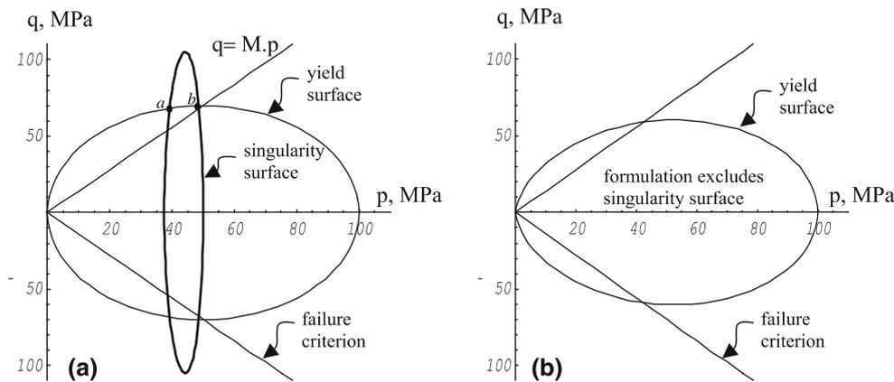
**Fig. 6** Various surfaces in stress space of **a** Model 8 and **b** Model 1 (parameters:  $G = 10$  MPa,  $\kappa^* = 0.02$ ,  $\lambda^* = 0.2$ ,  $M = 1.4$ ;  $p_{c0} = 100$  MPa)
