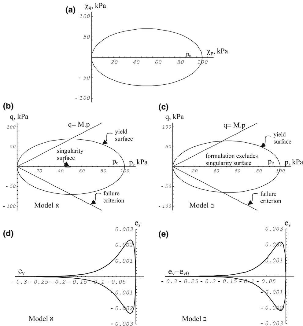
**Fig. 5** a Yield surface in dissipative stress space for both Models 8 and 1. b and d gives the stress, and strain space projections of the yield surface in Model 8, while (c), and (e) gives
