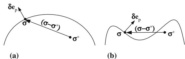
**Fig. 1** **a** Convexity and **b** concavity of yield surfaces in strain space
