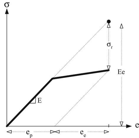
Fig. 3 Decompositions of strains ( $e = e_e + e_p$ ) and stresses ( $\sigma = Ee - \sigma_r$ ) in linear-elastic/plastic models
