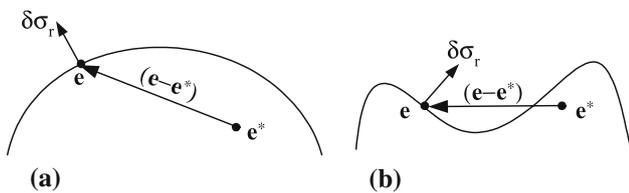
Fig. 2 a Convexity and b concavity of yield surfaces in strain space
